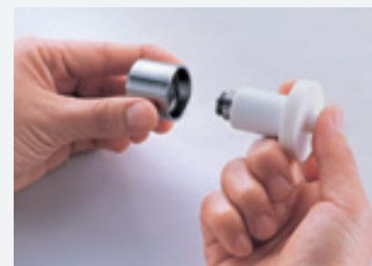
**To dismantle**, push unit collet + nut into the collet extractor in order to squeeze the collet. Remove the nut.
