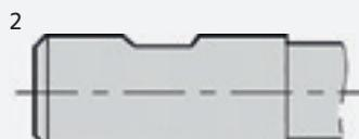
DIN 1835 B/DIN 6535 HB up to Ø 20 mm
