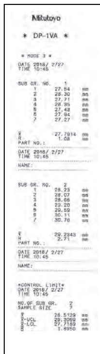
Mode 3 N: Number of data MAX: Maximum value MIN: Minimum value n: Number of subgroup (Max.10) X: Average value of subgroup R: Range of subgroup X̄: Mean value X-UCL: Upper control limit R: Mean (R control) R-UCL: Upper control limit (R control) R-LCL: Lower control limit (R control)
