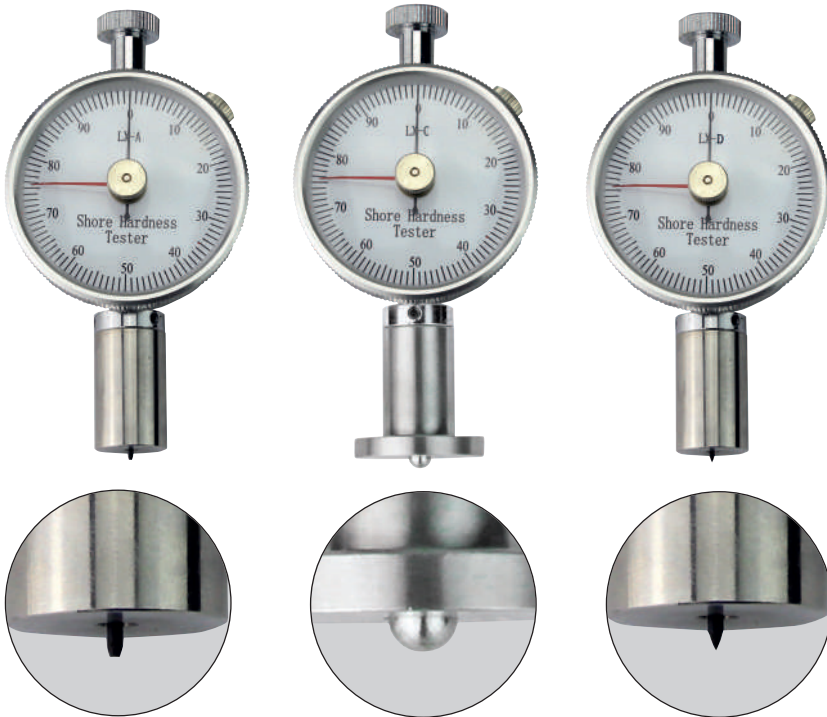
A: Flache Kegelspitze (ø 0,79 mm), 35° Flat cone point, (ø 0.79 mm), 35°
