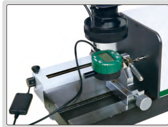
check INSIZE digital indicators (connection with cable)
