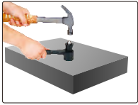
hammer impact to apply test force
