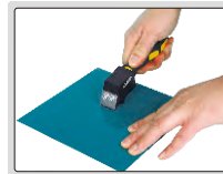
step 1: make grid cutting on surface
